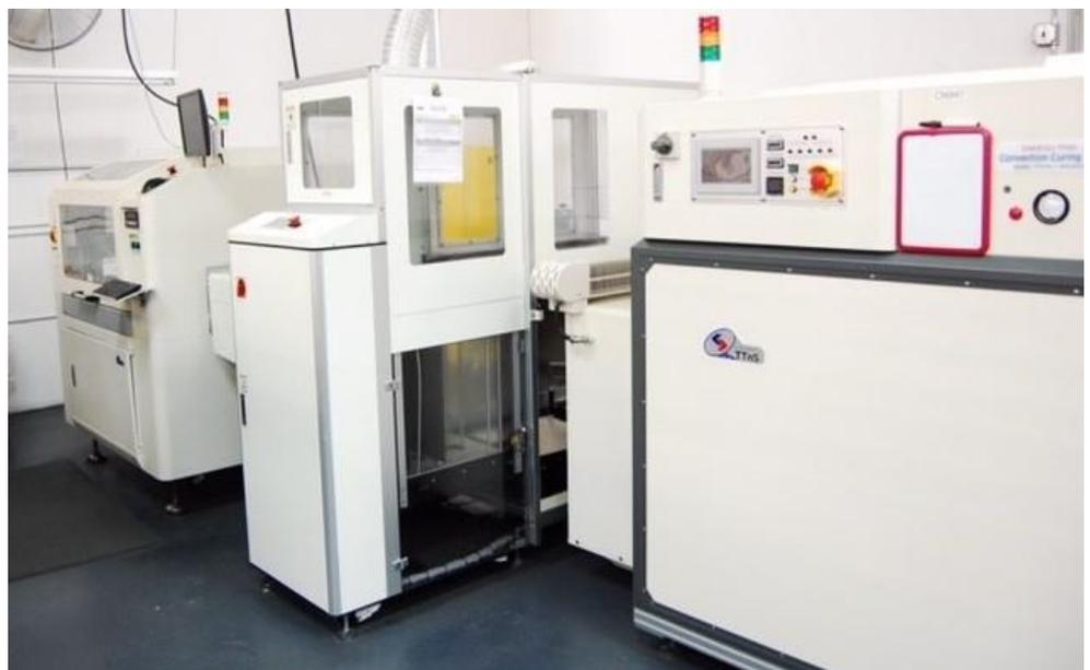
SoPark's robotic selective coating system with large 15.75 in. X 22.0 in. capability.
